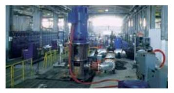
We recently achieved the important objective of fitting every Unit with a modern Testing Room: in our plants in Gessate and S. Mauro Torinese we can test pumps with powers up to 650 kW, capacities up to 8000 m3/h and pressure values up to 120 bar. Our plant in Taglio di Po has been designed for sealless pumps intended for applications in the chemical sector.
